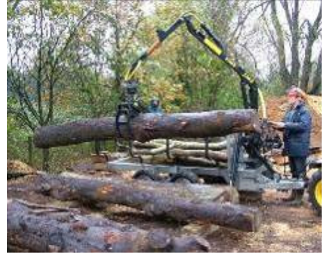
HIGH LIFT CAPACITY CRANES: 700-1000Kg UP CLOSE AND 340-400Kg AT FULL REACH.
