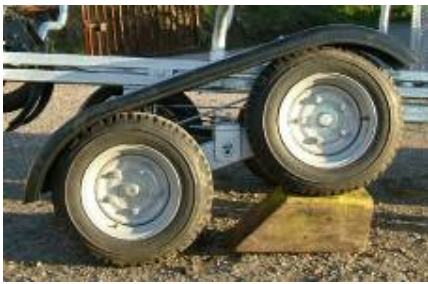
HIGH CLIMBING ANGLE, ROCKING BEAM AXLES WITH LEAF SPRING SUSPENSION FOR SMOOTH RIDE.
