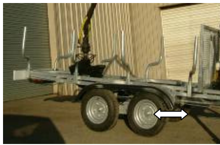
HYDRAULICALLY ADJUSTABLE BED ALLOWS YOU TO MOVE THE AXLE TO ENSURE THE LOAD IS POSITIONED TO ENSURE THE NOSE WEIGHT DOES NOT EXCEED THE LEGAL LIMITS. WHY RISK YOUR SEFETY AND YOUR LICENCE!
