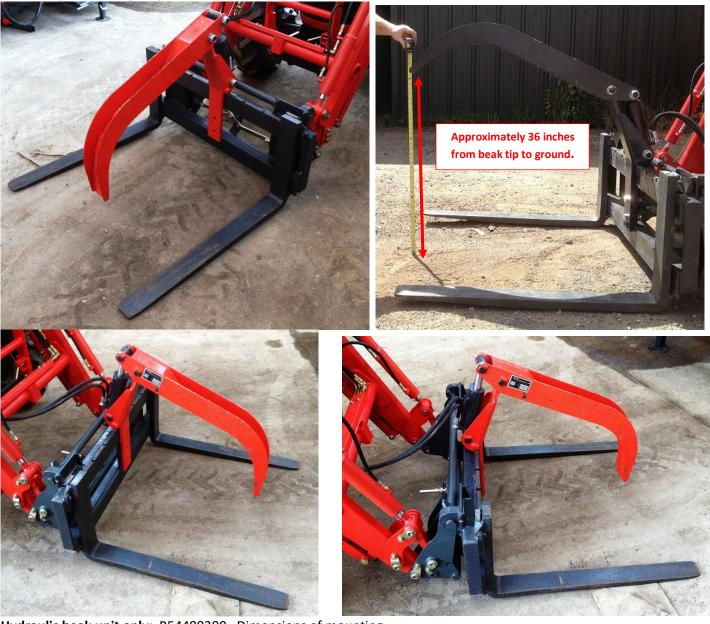
Hydraulic beak unit only: R54480200. Dimensions of mounting.
