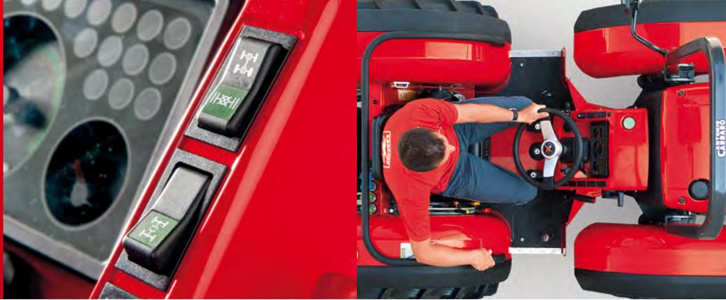
The elegant and intuitive on-board instrumentation includes an anti-glare screen with backlighting for night use and an "on-off" information system. All the electro-hydraulic controls are button-controlled and within easy reach.
