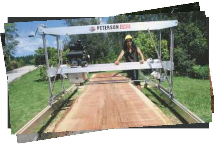
Peterson's [Dedicated Wide Slabber](#) (DWS) is not a swingmill like the rest of the range; its sole purpose is to cut logs into wide slabs.
