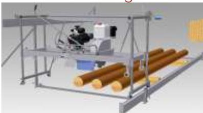
Mill multiple small logs at a time on one set of skids to increase productivity.
