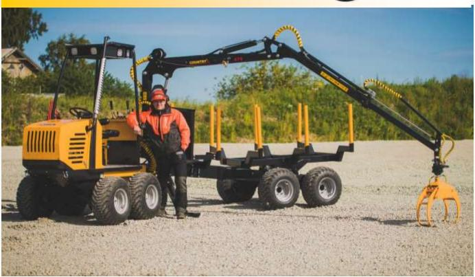
The Kinetic has been designed as a serious, high output, professional machine for low impact work by forestry owners and contractors. The standard build includes crane grab and rotator and the hydraulic extending chassis to reduce the length for transport to 5187cm from the working length of 5787cm.
